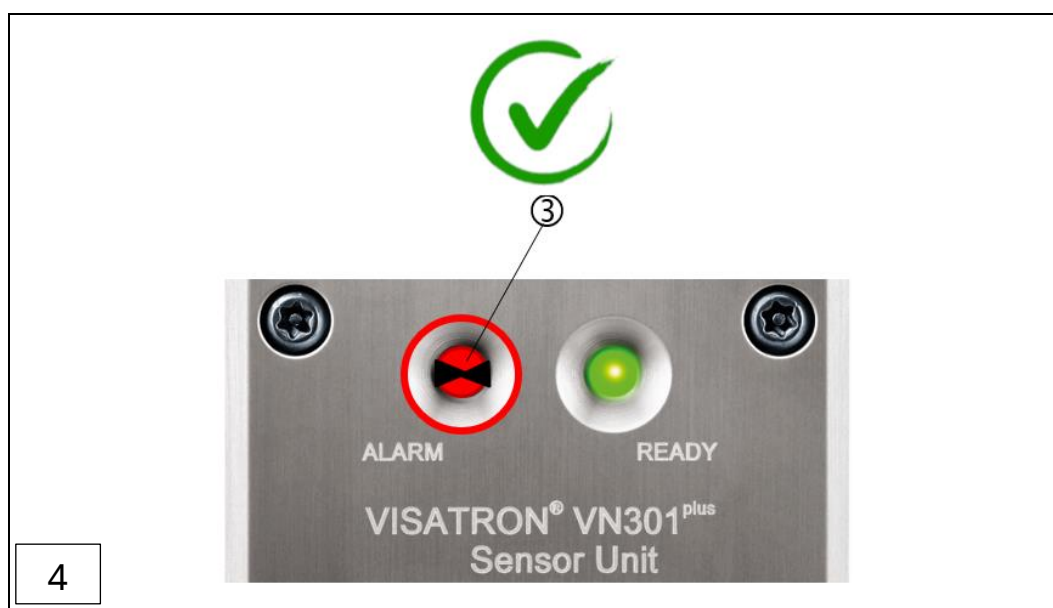
Fig.: 84 : Function test with smoke tube (mist test, steps 1-4)
