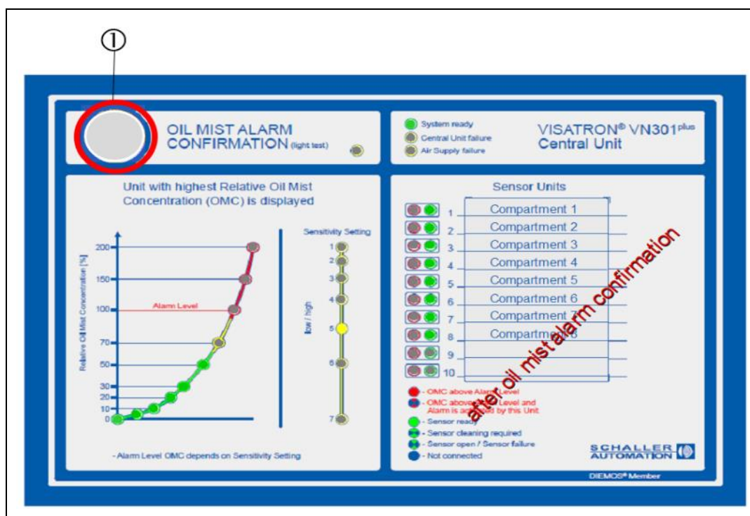
Fig.: 89 : VN301 plus central unit: Status indicator after confirming the oil mist alarm
