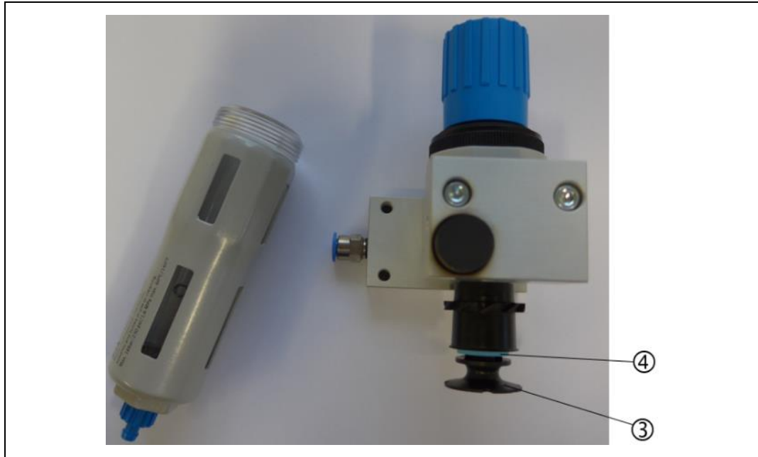
Fig.: 95 : Replacing the air filter element, pressure regulator unit
