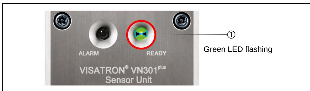
Fig.: 103 : VN301 plus / VN301 plus EX sensor unit: “Ready” status LED indicator
