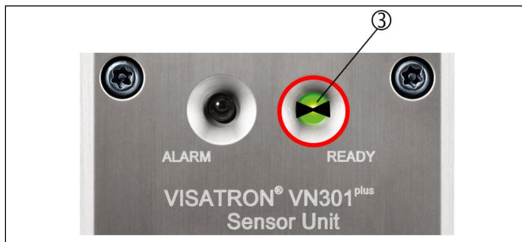
Fig.: 91 : "Sensor cleaning" status indicator on the VN301 plus / VN301 plus EX sensor unit
